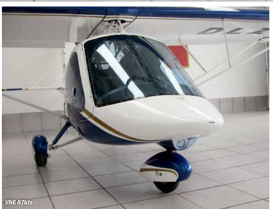
Built with alloy 6061-T6 aluminium tubes
