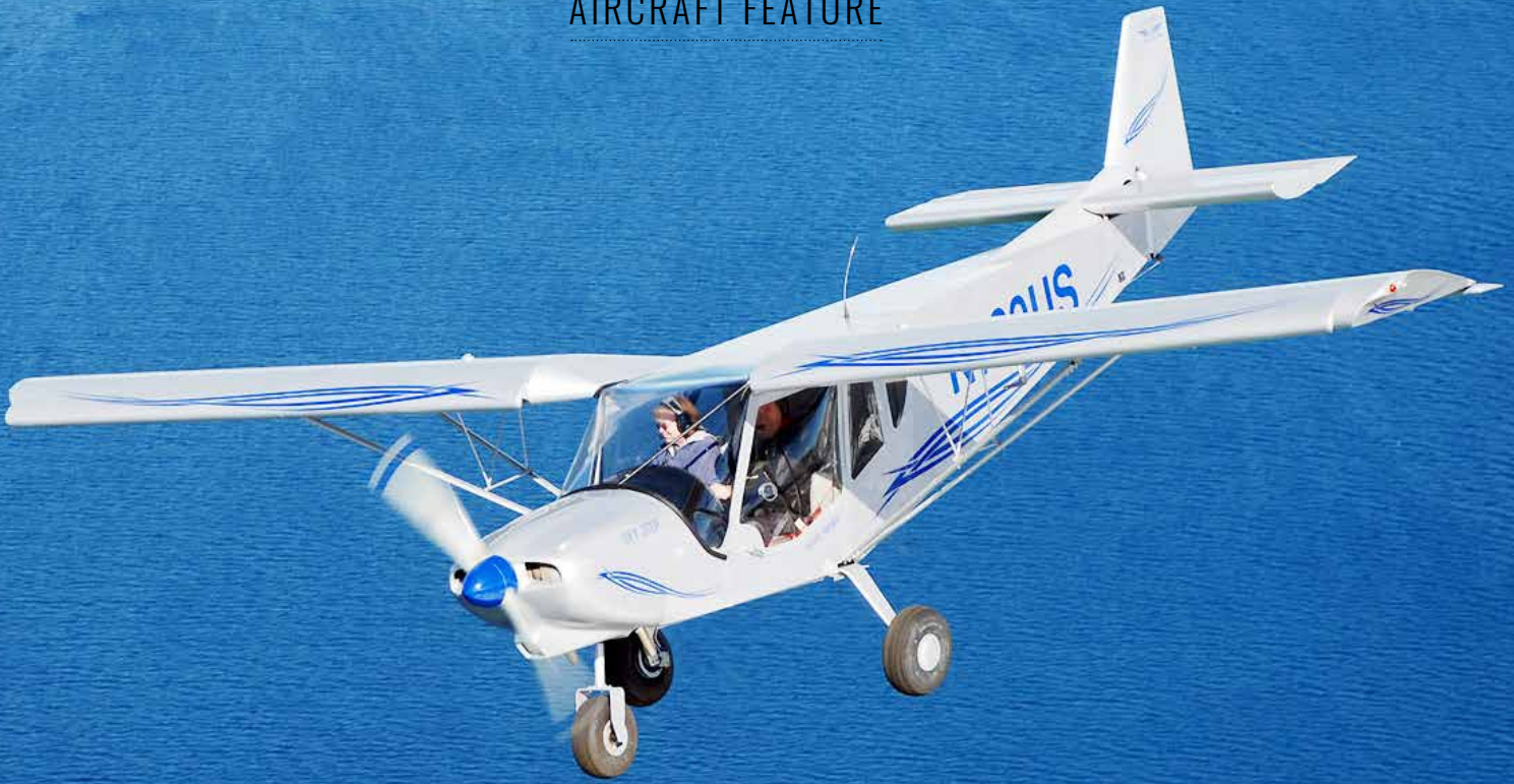
New raised skylight and increased cabin height
