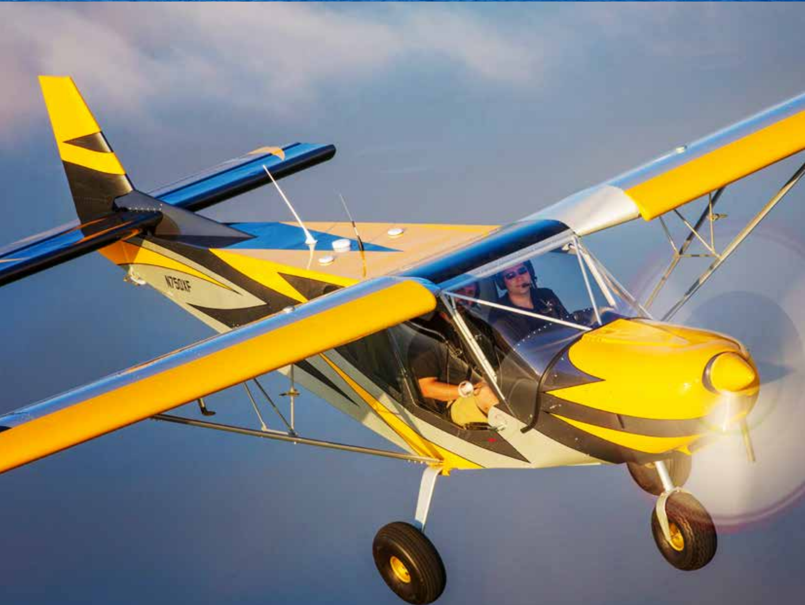
Full length flaperons and all-flying rudder
