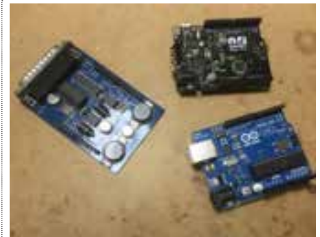
A genuine Arduino, a clone and a home brew EGT-CHT Arduino shield
