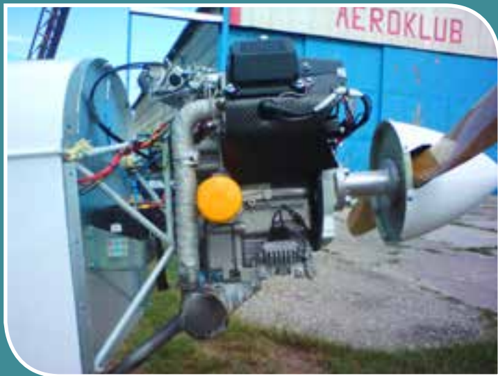
>> The Kohler CH750 installed in the factory demonstrator. The engine receives only a few modifications: removal of all the metal shrouds and fan, lightening of the flywheel, relocation of the carburettor and a new intake manifold and air ducts. The prop is attached to an extension bolted to the flywheel.
