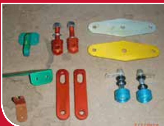
>> The 51% kit also contains all controls, ready to paint. I have experimented with anodising the aluminium parts and have achieved some nice results. Anodising is a substitute for aluprep and paint or alodine to protect the aluminium parts from corrosion.
