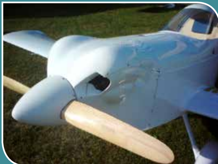
>> The Kohler CH750 installed in the factory demonstrator. The engine receives only a few modifications: removal of all the metal shrouds and fan, lightening of the flywheel, relocation of the carburettor and a new intake manifold and air ducts. The prop is attached to an extension bolted to the flywheel.
