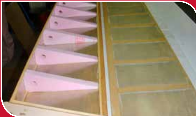
>> A flaperon before closing. After putting the skins on, the pre-formed leading edge foam is glued on and covered with fibreglass to provide some impact resistance. The rudder, fin and main wings are built in a similar way.
