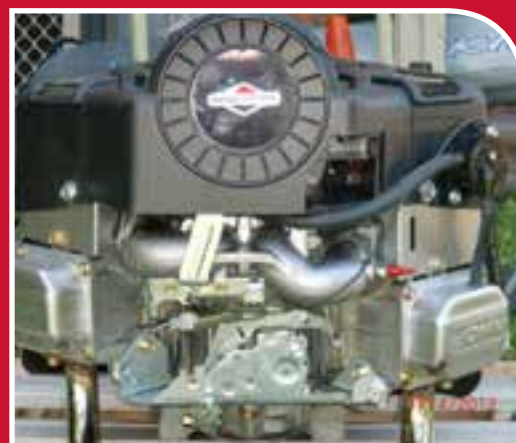
>> The engine still needs to be converted for aircraft use. It will be installed as a hanging V with a dry-sump oil system a la Rotax 912 (using blow-by to pump the oil from the engine to the oil tank).
