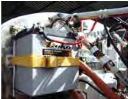
>> The Arion Lightning was fitted with a larger battery to insure against a lack of power
