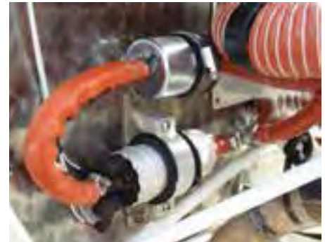
>> A high pressure pump and quality fuel filter fitted very neatly on the firewall
