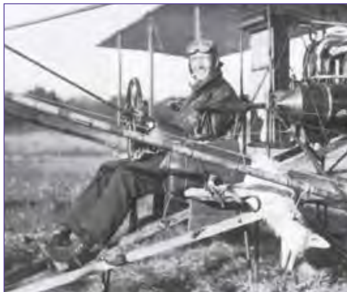
>> Glenn Curtiss in the Rheims Flyer-1909 - the cushions against his shoulders are the aileron control yoke.
