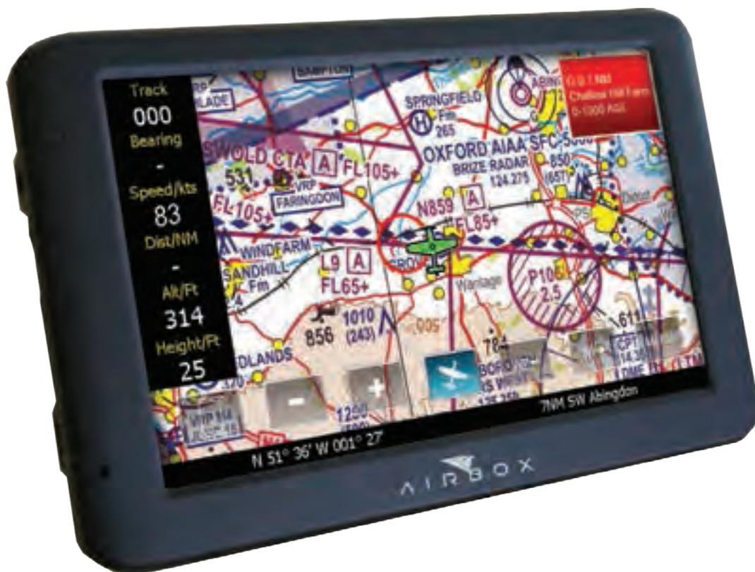
variable distance extension indicator telling you where you're expected to be up to ten minutes ahead. Alternatively, this can also be used to line-up on a long final as an extended runway centre line. Once you move outside the limits of the VNC you have been using, the unit automatically changes the chart view to WAC, seamlessly maintaining position & scale.
