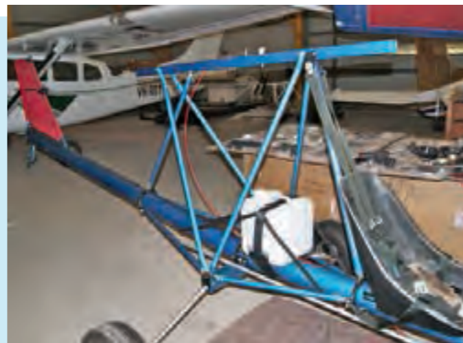
STAGE 5 Attachment of the rear tube to the main body. Align, measure and check it is square to the front tube. Attach and adjust elevator controls. Also attach fuel tank straps and the flap handle controls, which will be on the main tube (like the GT500) instead of the root tube, due to the option of the wing tank.
