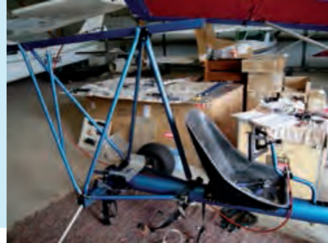
STAGE 2 Assembly of the seat and seat track, control wheel, extra fuel tank bracket, front wheel assembly and rudder pedals. (This has the optional Quicksilver GT500 front wheel assembly)
