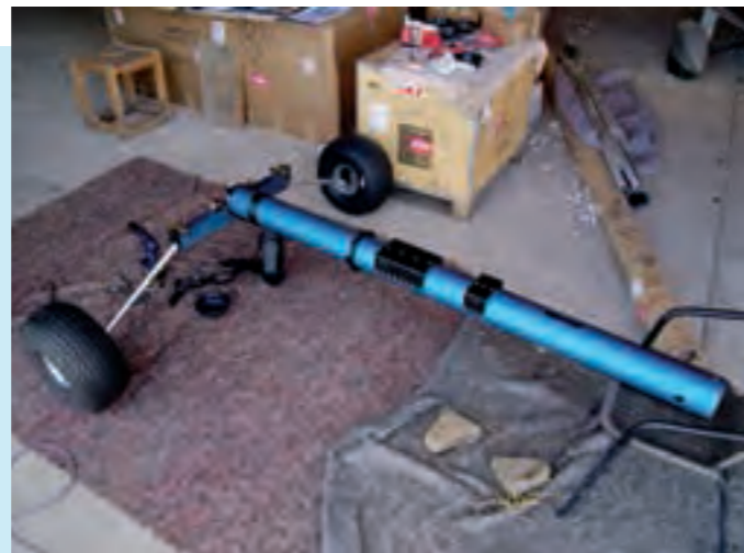
STAGE 1 Assembly of the forward tube, axles, brake and wheel assembly. (This has the optional Black Max brake system and optional tundra tyres)
