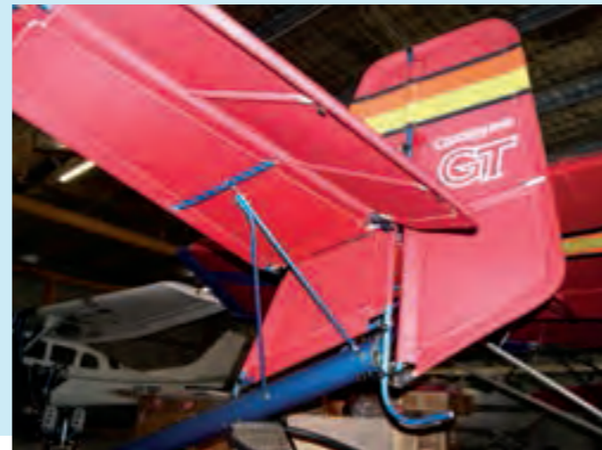
STAGE 3 Assembly of the root tube, aileron control and cabin frame.
