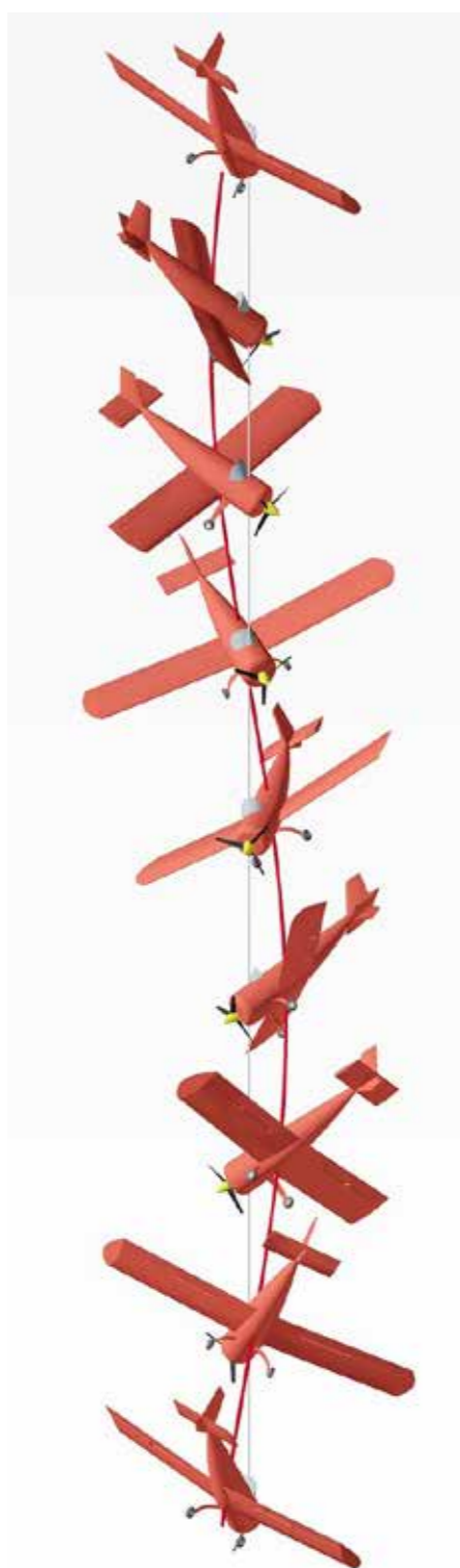
Figure 1 - A fully developed spin - the aeroplanes centre of gravity follows a corkscrew path around a vertical axis.
